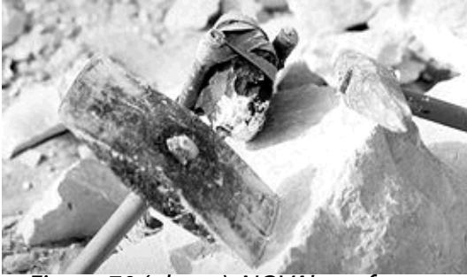
Figure 70 (above): NOVA's craftsmen used modern steel tools (left and right), not the Old Kingdom stone tool imitation (center).
