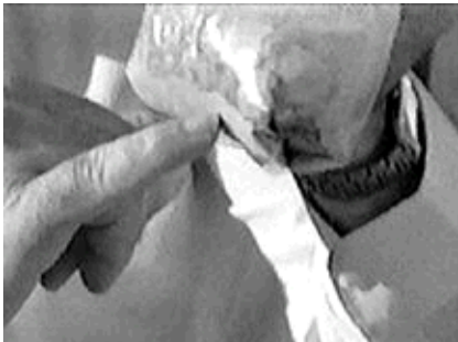
After 24 hour soaking in a plastic bag with water, the limestone chunk separated into clay and nummulites. In the presence of an excess of water, the heavier clay settles, leaving the nummulites separated from each other. "This Old Pyramid" WGBH, Boston, 1992.
