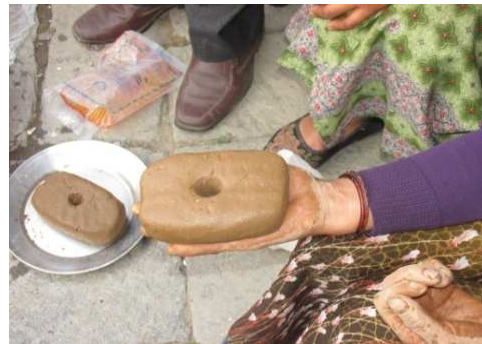
Fig. No. 3.1.7 Making rectangular shape, and small hole in center Source: JICA Project Team
