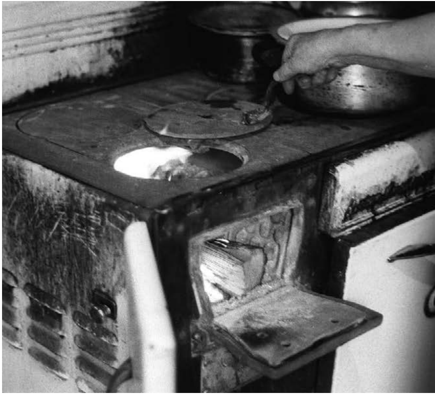
All the eyes on the stove can be removed with the lifter, a tool that comes with most wood cookstoves.
