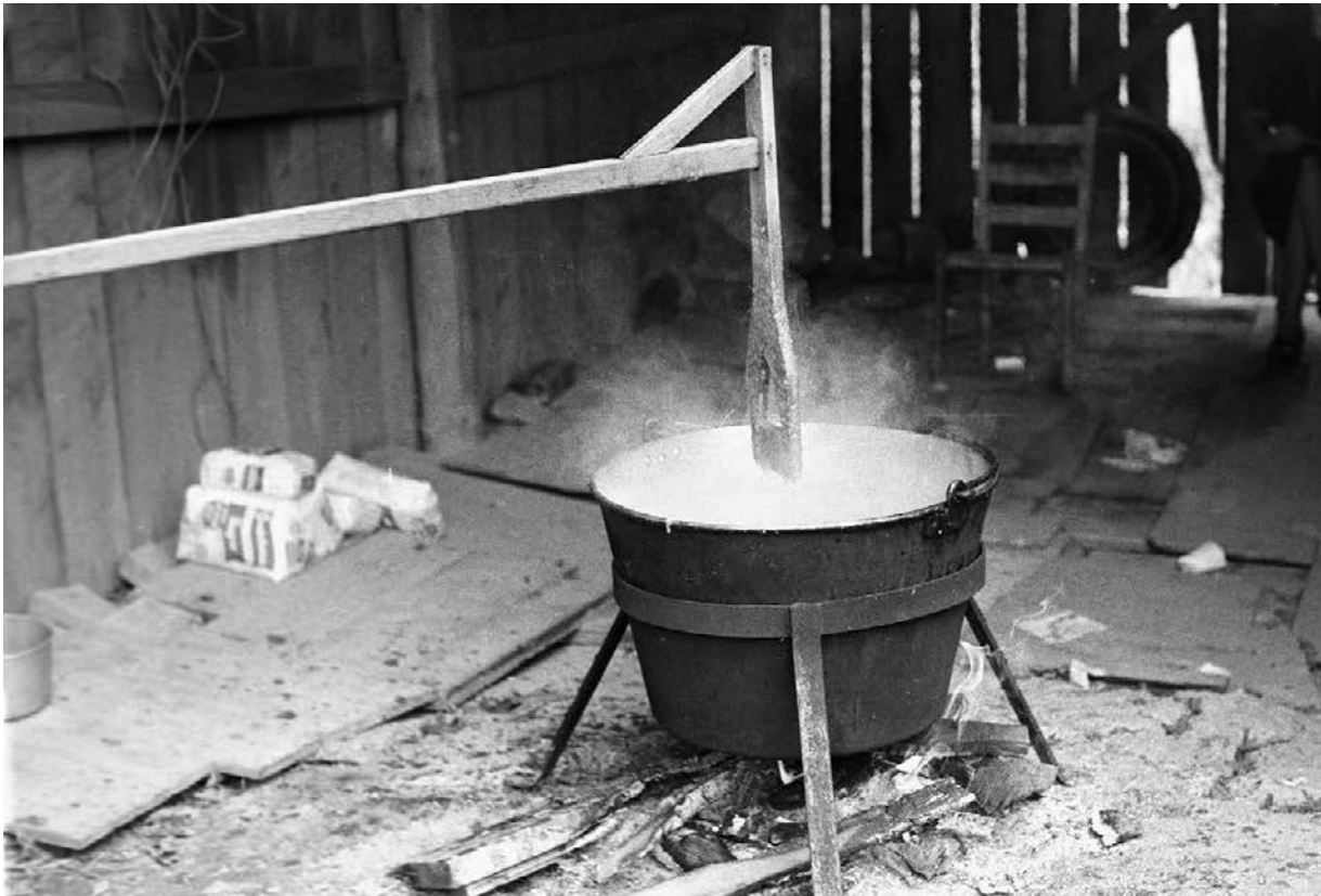
Mr. Brooks made the butter-stirring stick out of cypress. Wood with acid in it can't be used because it will taste. He likes yellow poplar the best.
