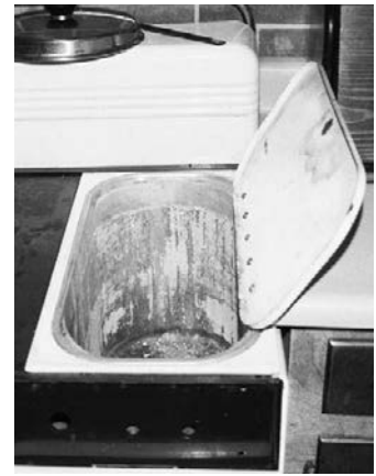
Two views of an enamel-lined reservoir.
