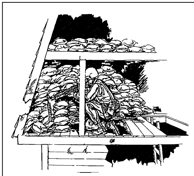
Figure A-66. Firing Platform Built Under a Roof
