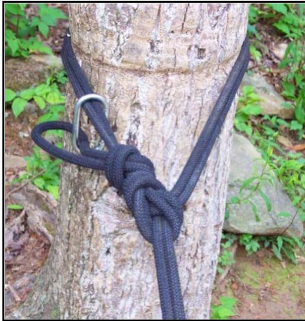
Figure 5-10. Rope tied to anchor with anchor knot.
