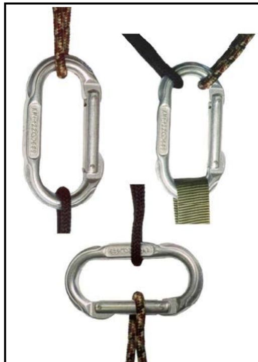
Figure 3-12. Major and minor axes and three-way loading.
