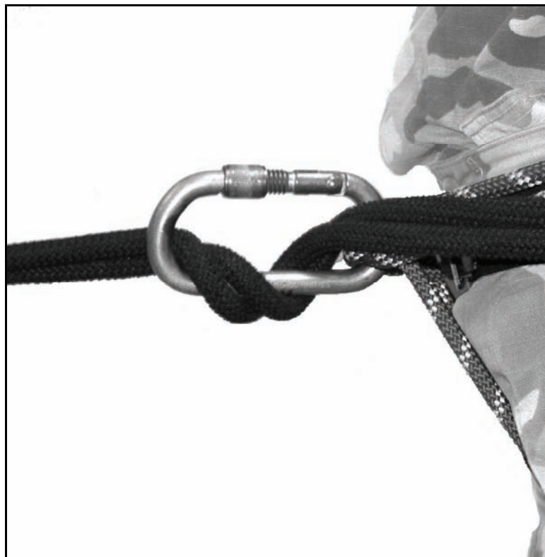
Figure 2-8. Proper hookup using carabiner wrap.
