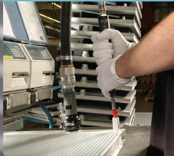
Tightness testing on the finished product.
