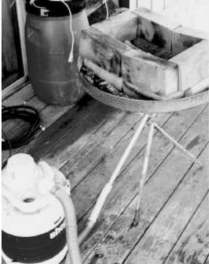
Assembled forge with shop-vac
