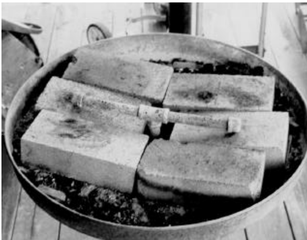
Placement of the bottom bricks and tuyere
