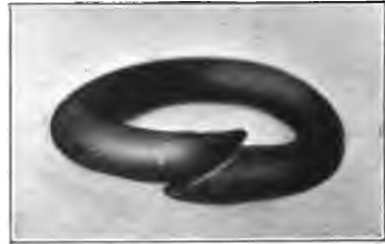
FIG. 37. SHOWING SCARFS ON LAP WELD OF RING.
