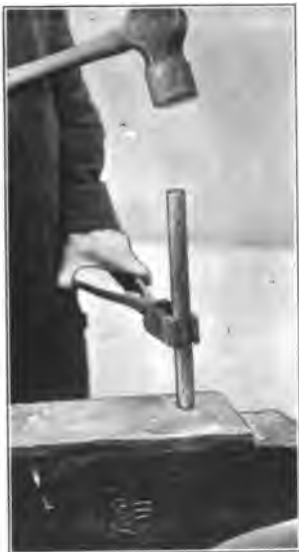
FIG. 12. SQUARING AN END, ALSO UPSETTING.
