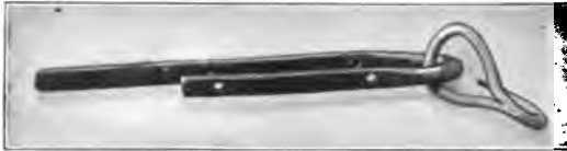
FIG. 49. SINGLE TREE HOOK AND STRAP.
