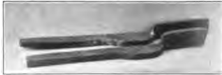
FIG. 57. TWO JAWS OF HOOF PARERS.
