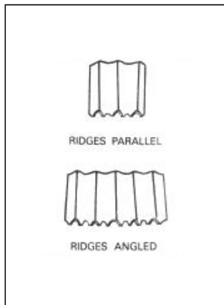
**Figure 2-16. Corrugated fasteners**
