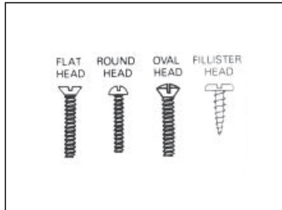
Figure 2-10. Sheet-metal screws
