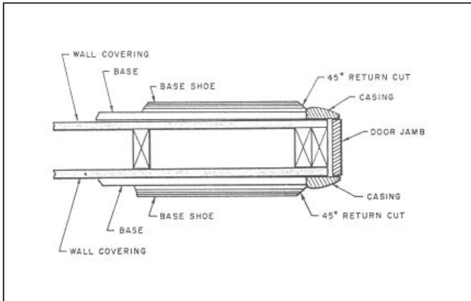
**Figure 9-9. Base-shoe trimming**
