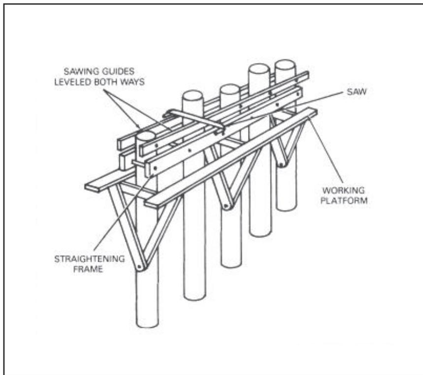
**Figure 11-7. Cutting piles**
