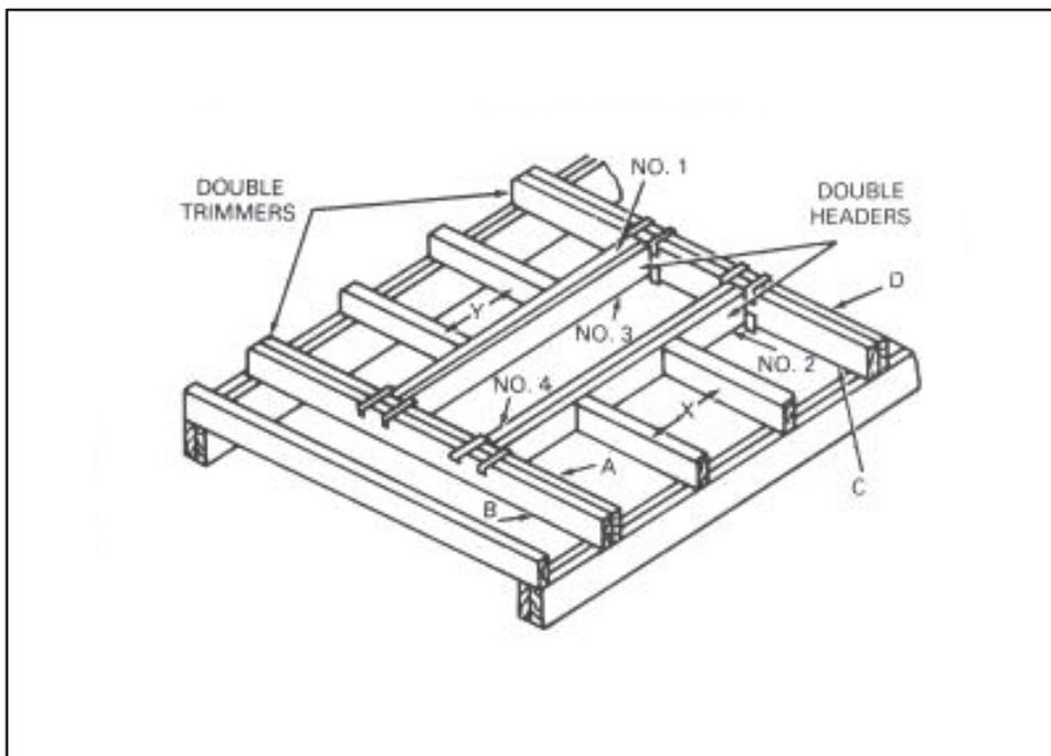
**Figure 6-25. Floor-opening construction**
