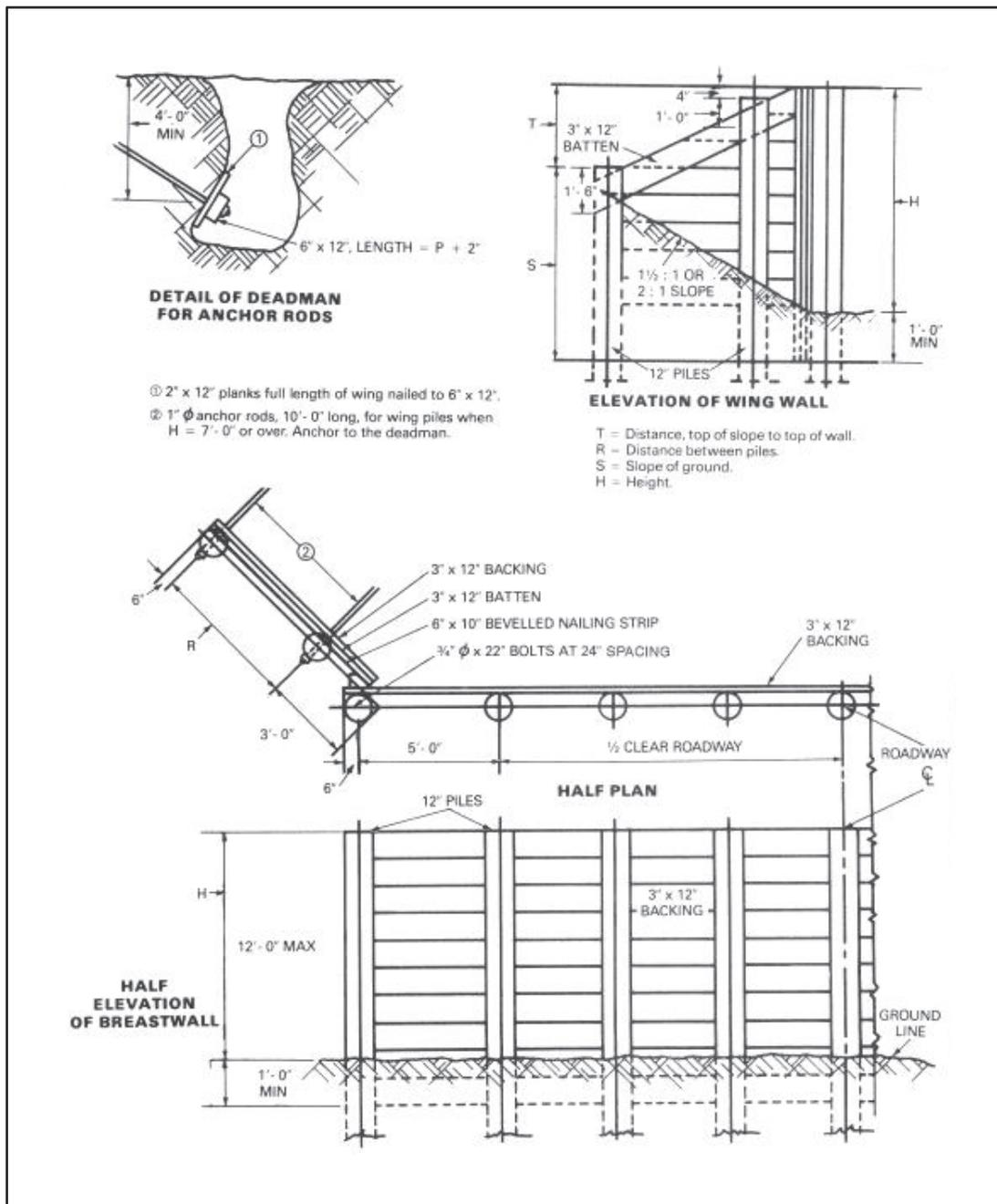
Figure 10-11. Retaining-wall details
