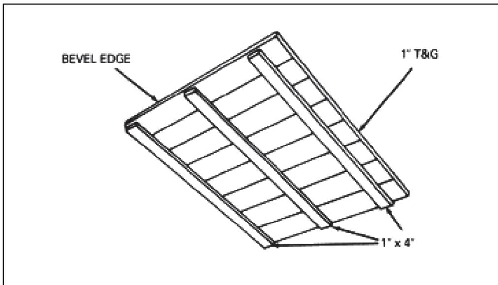
Figure 5-14. Floor slab form
