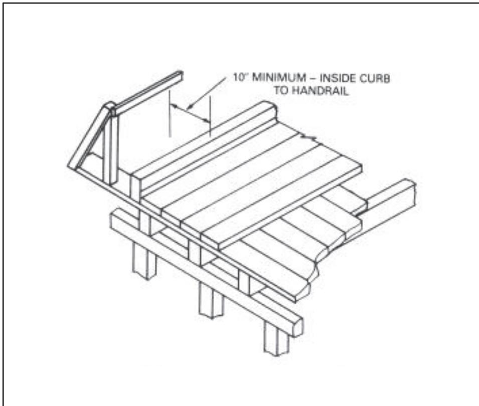
Figure 10-17. Solid-plank deck
