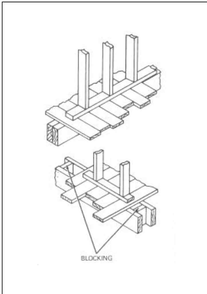
Figure 6-19. Reinforced joists
