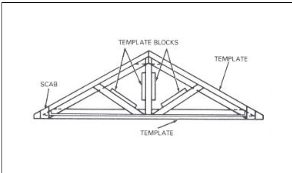
Figure 7-21. Temporary bracing
