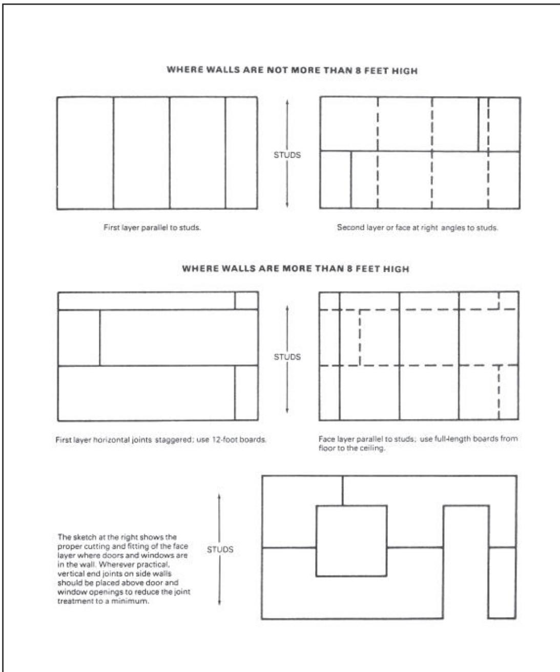
**Figure 9-1. Hanging sheetrock and wood panels**
