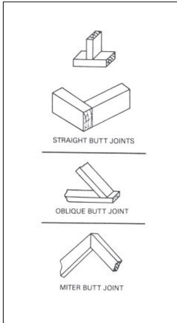
**Figure 6-4. Butt joints**
