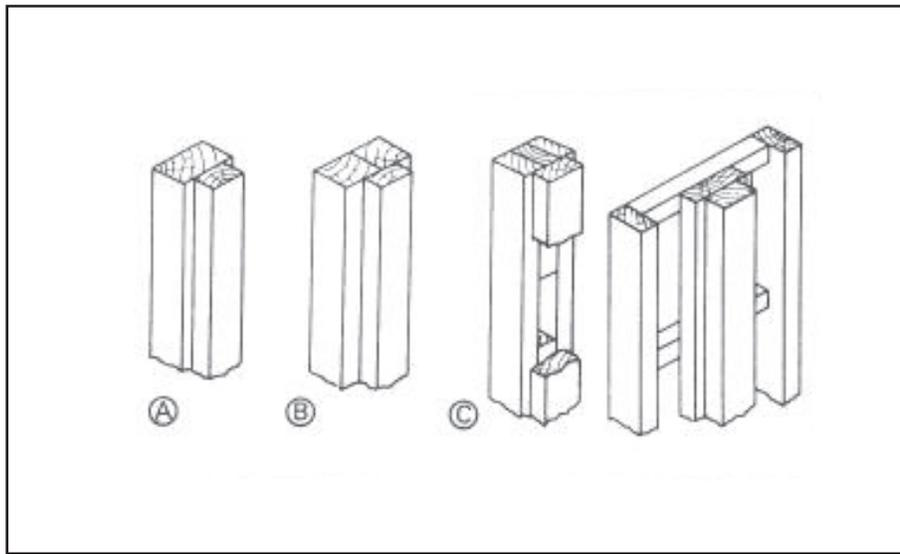
Figure 6-33. T-Post construction
