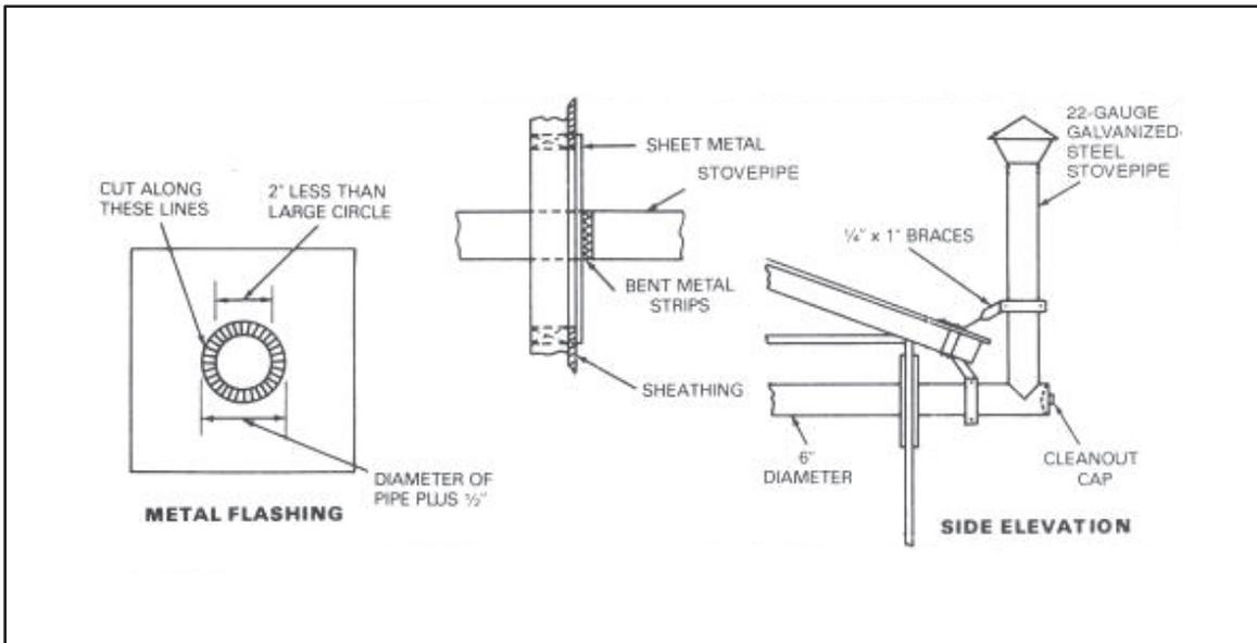
Figure 6-48. Installing stovepipe
