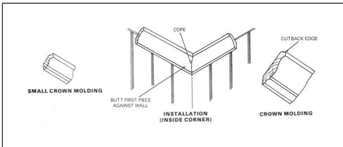
Figure 9-12. Ceiling molding
