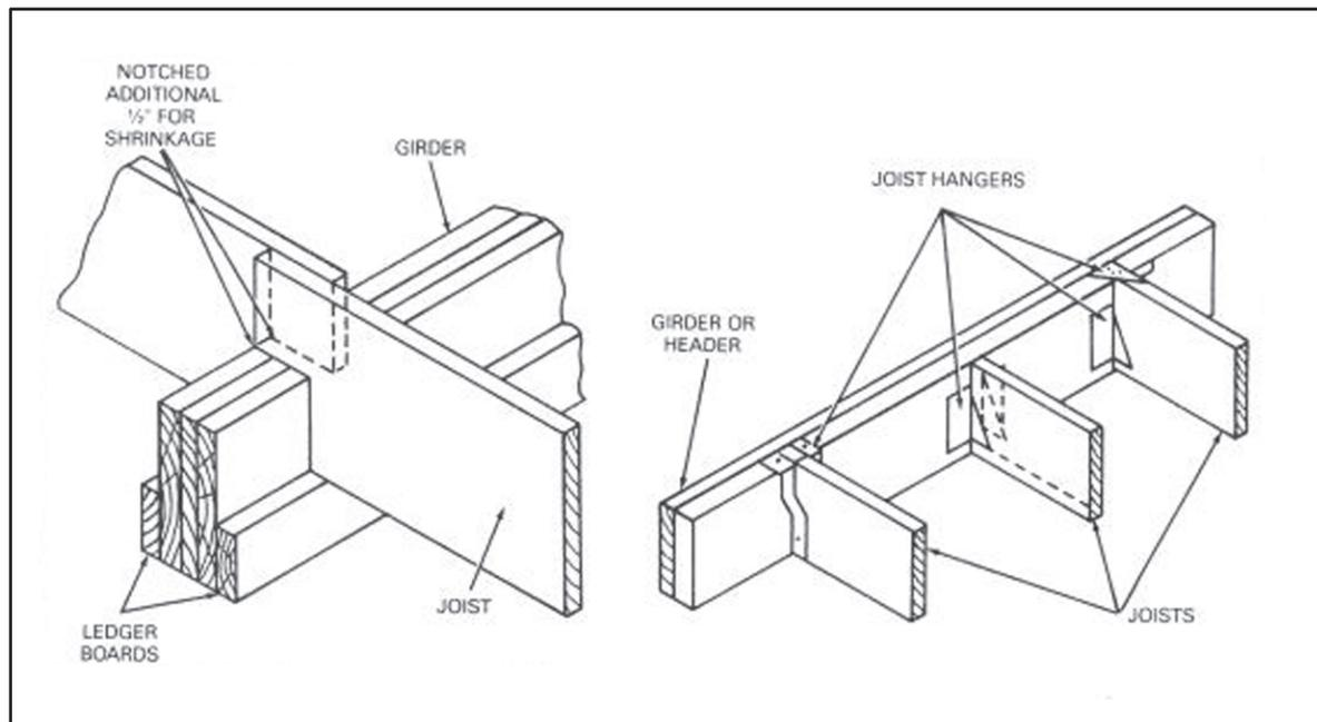
**Figure 6-11. Joist-to-girder attachment**
