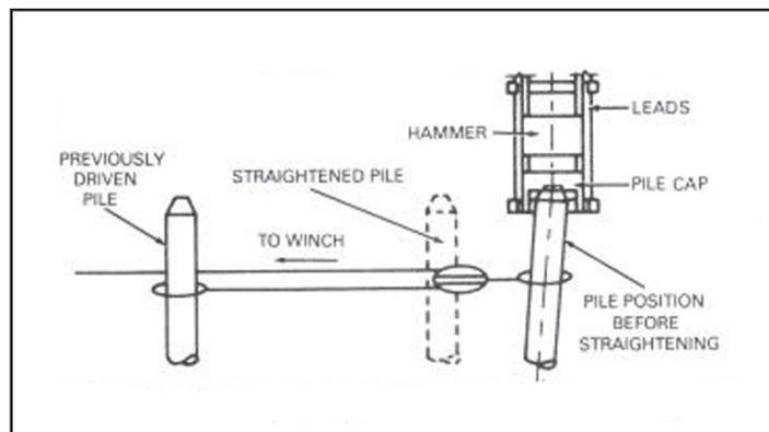
Figure 11-3. Realigning with a block and tackle
