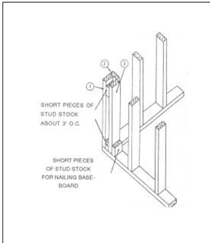
Figure 6-31. Alternate corner-post construction using ordinary 2 x 4 studs
