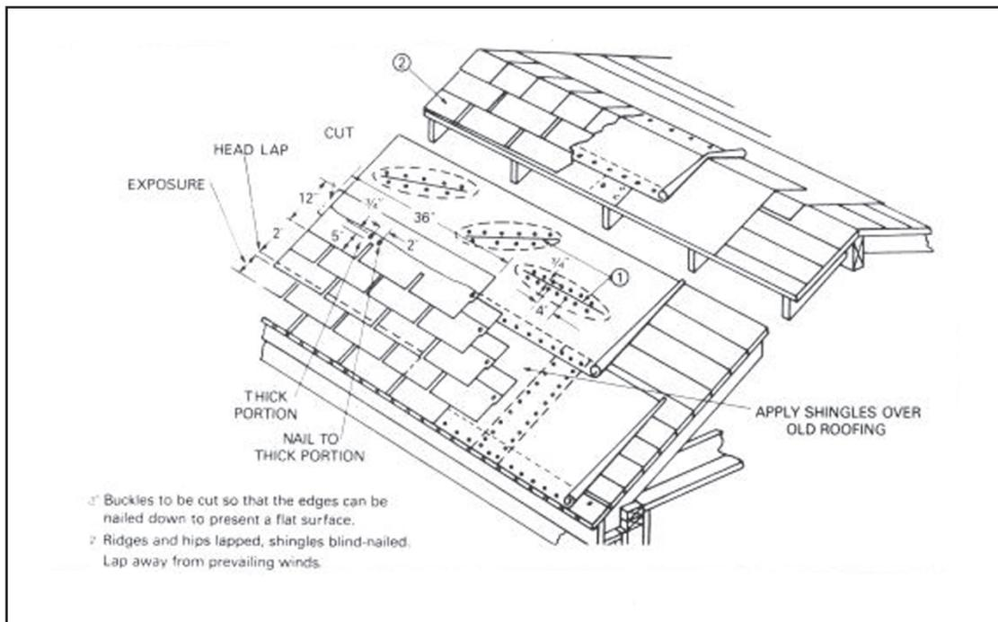
**Figure 7-30. Roof replacement**
