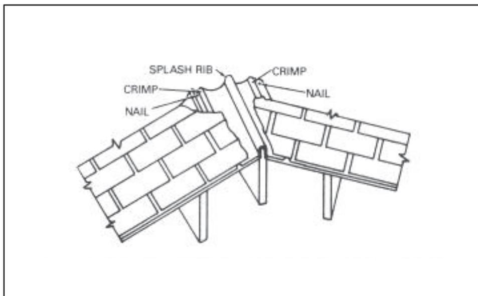
**Figure 7-27. Open-valley flashing**
