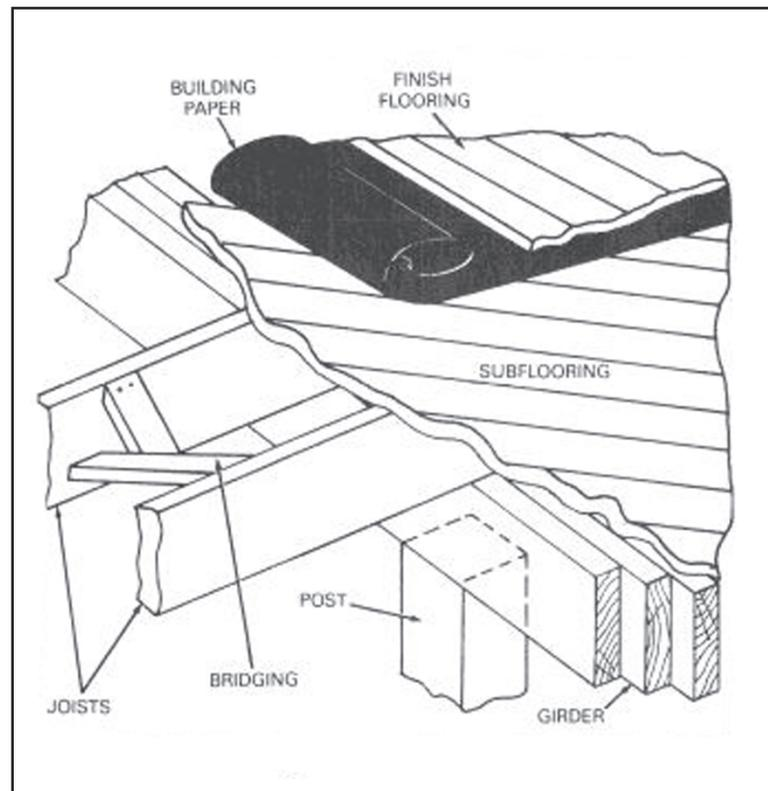
**Figure 6-18. Floor joists**
