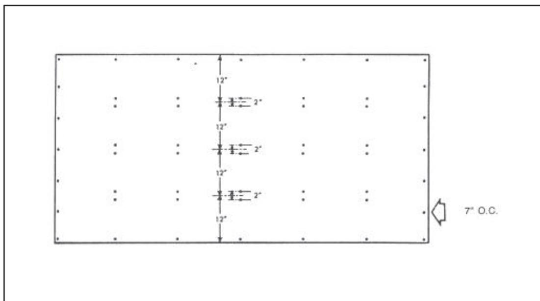
**Figure 9-4. The double-nailing system for installing sheetrock**
