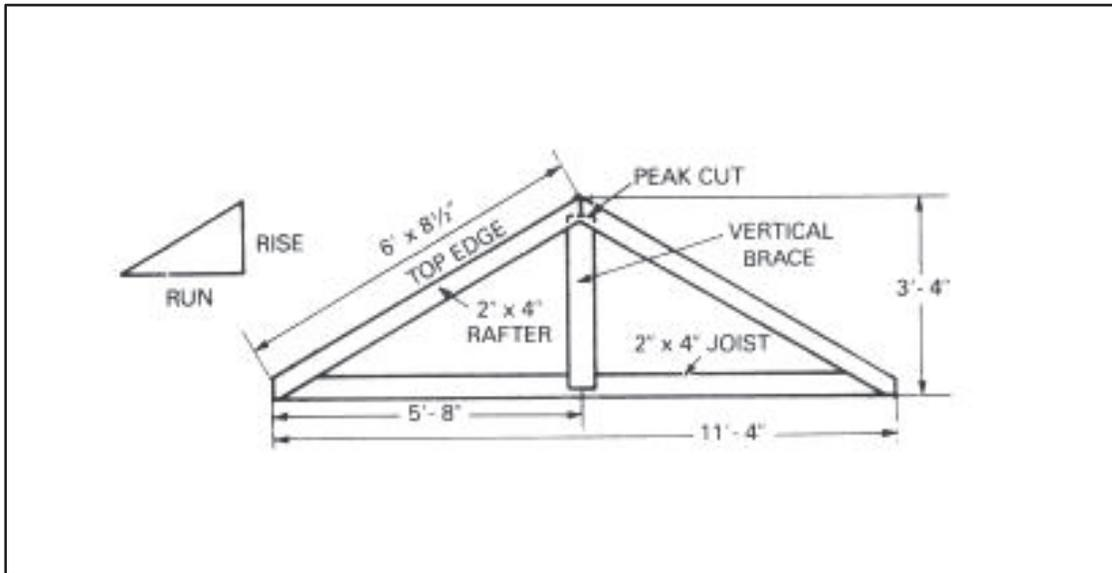
**Figure 7-15. Truss layout**
