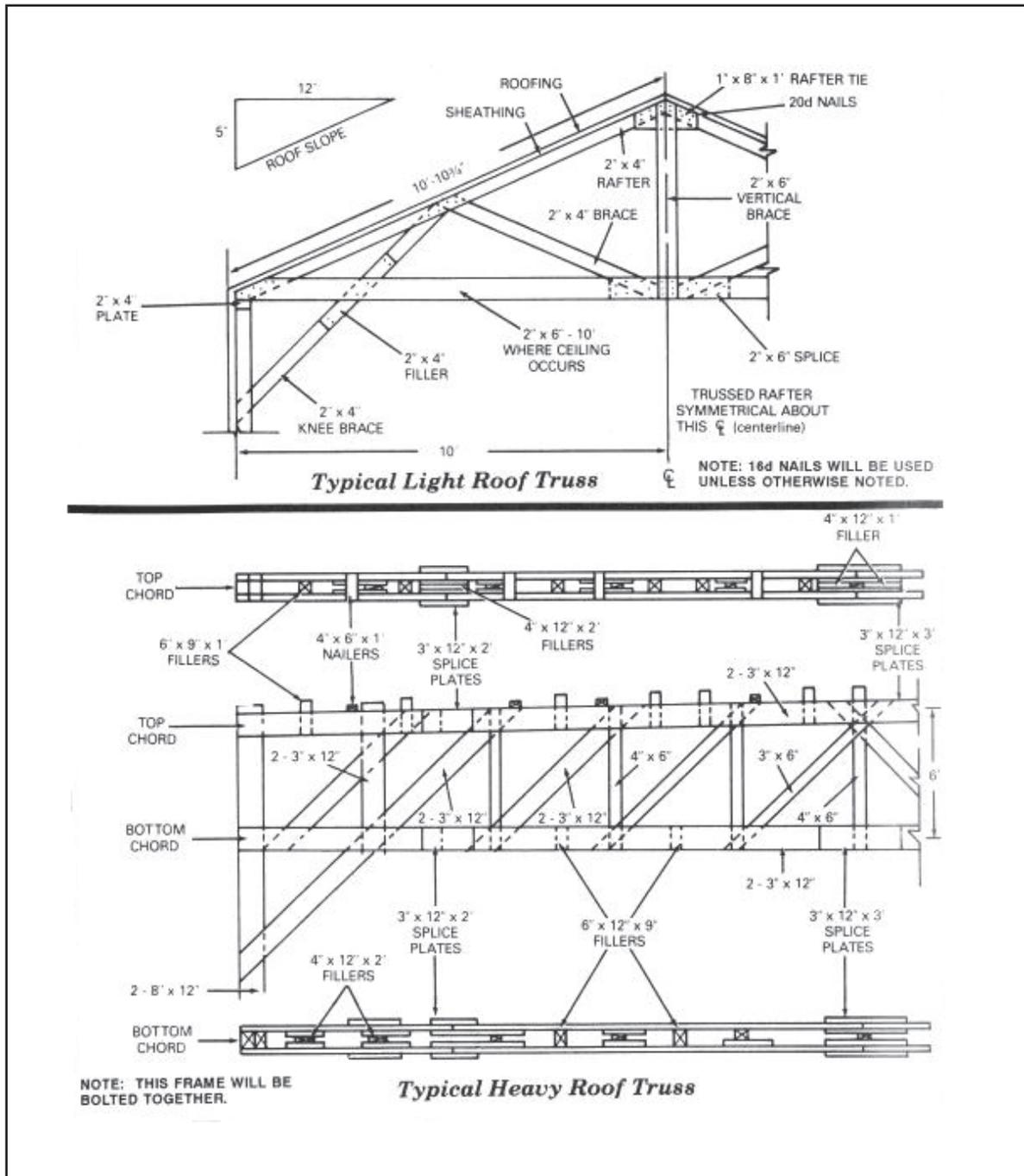
Figure 1-18. Roof trusses
