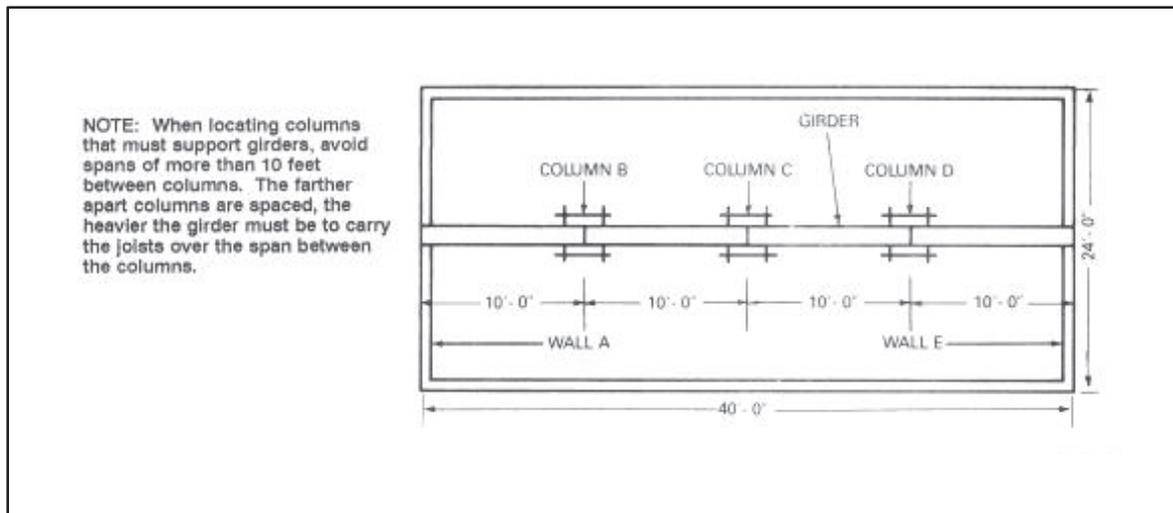
Figure 6-16. Column spacing
