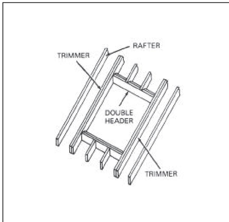
Figure 7-22. Roof-opening construction
