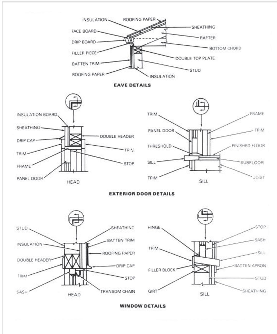
Figure 1-10. Typical eave, door, and window details
