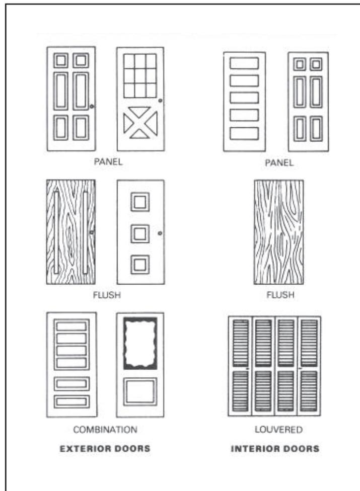
**Figure 8-2. Mill-built doors**
