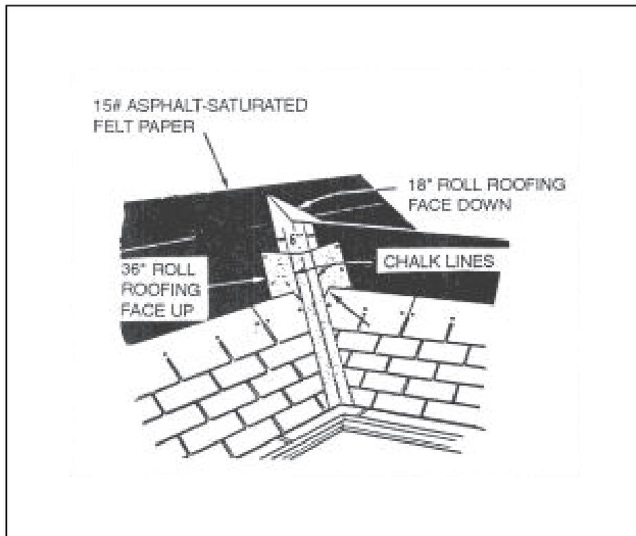
**Figure 7-31. Open-valley flashing**
