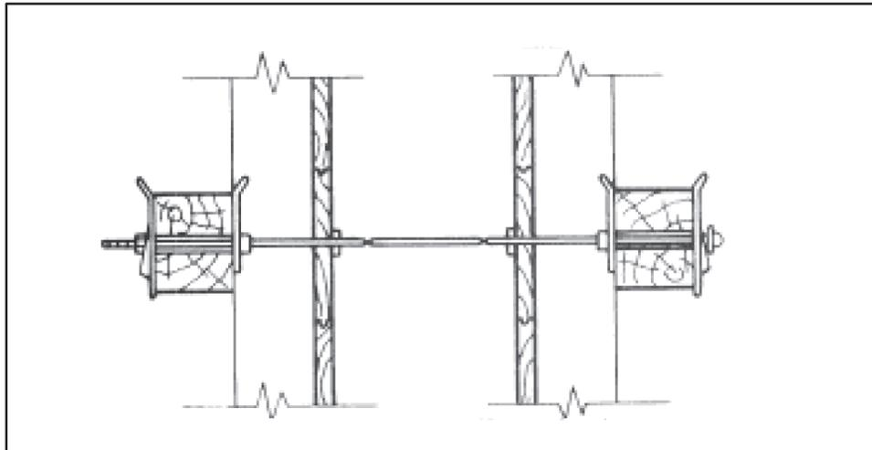
Figure 5-9. Tie rod and spreader combination
