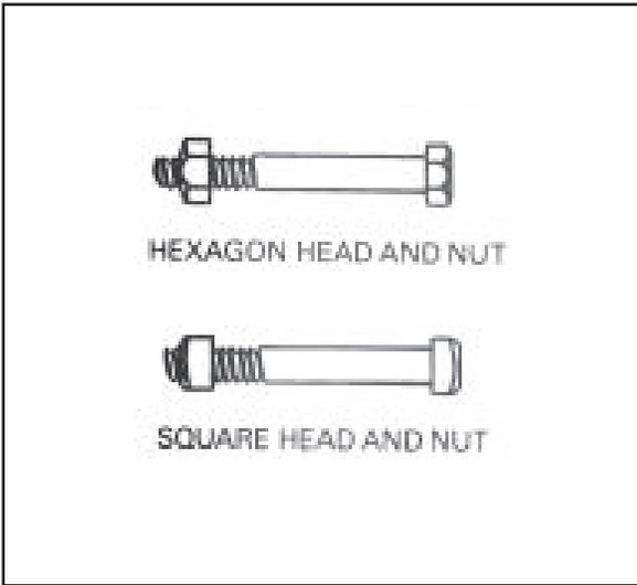
Figure 2-12. Machine bolts
