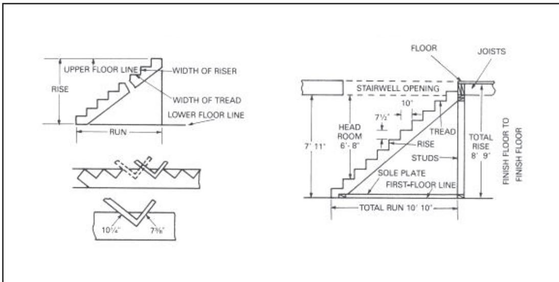
Figure 6-51. Step construction
