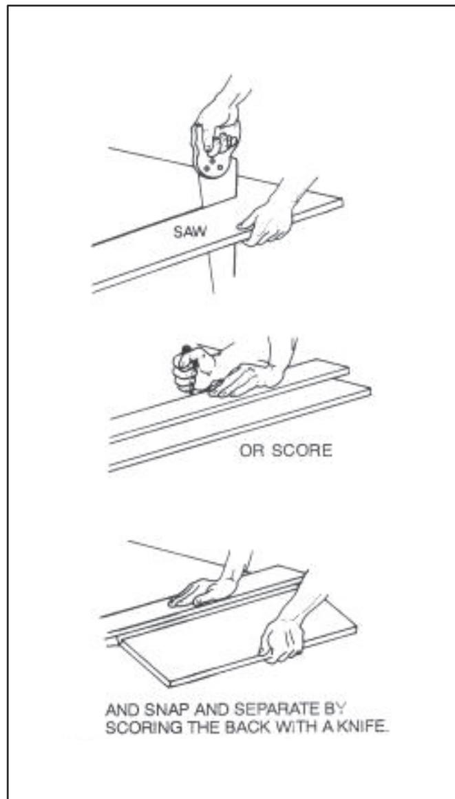
**Figure 9-5. Cutting sheetrock**
