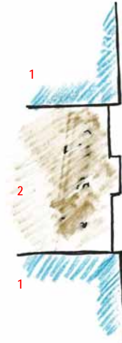
Figure 4.4: Bastard Tuck Jointing:
